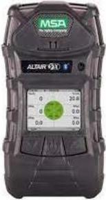
MSA has determined that PID sensors manufactured from March 2020 to and including June 2023 may not respond to gas after being turned on due to the lamp of the sensor not lighting upon startup and the Altair 5X PID will not display a PID lamp error. ***To verify proper operation of the Altair 5X PID, perform a bump test or manual gas check each time the unit is turned on prior to using the device.***
