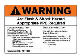
To achieve maximum safety, these labels should be installed on all existing enclosure doors, removable panels, etc. Per NFPA 70E 130.5 (H), labels must include the following information:
